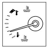
This gage shows the engine coolant temperature.
